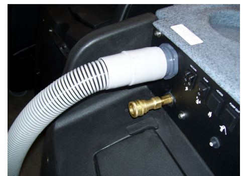
Vacuum Hose Connection with standard barb & vinyl cuff
