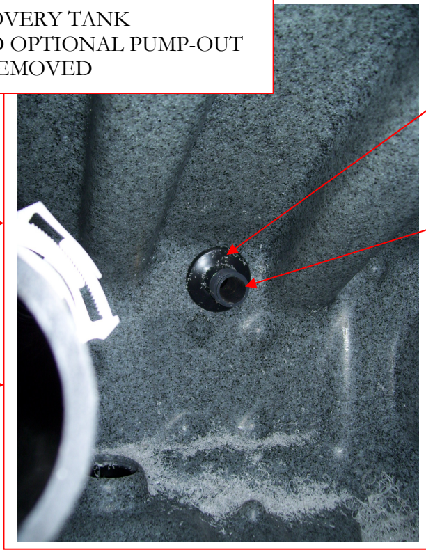
INSIDE RECOVERY TANK WITH OPTIONAL PUMP-OUT FILTER IN PLACE
