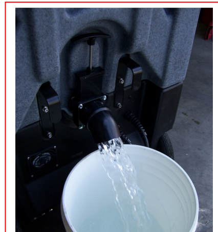
Drain water from Recovery Tank
